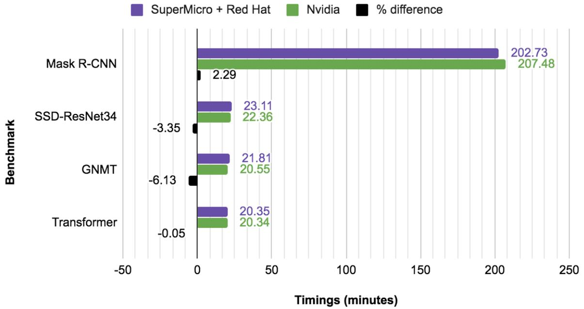
Figure 8: Benchmark results showing that MLPerf v0.6 on OpenShift was faster than the NVIDIA published timing for Mask R-CNN and only .05 to 6.13% slower for SDD-ResNet34, GMNT and Transformer.<sup>2</sup>
