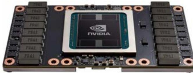
Figure 5: NVIDIA® Tesla® V100 SXM2 GPU
