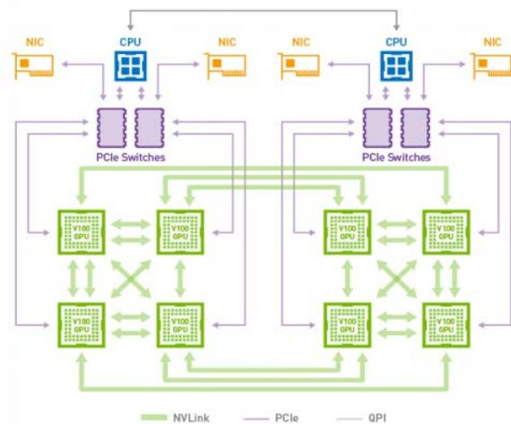
Figure 4: Hybrid Cube Mesh NVLink Topology
